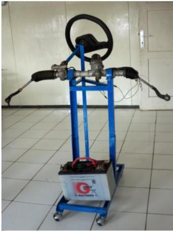
Gambar 3. Peraga Electric Power Steering
