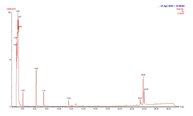
Figure 3. GC-MS chromatograph of the resulted furfural
