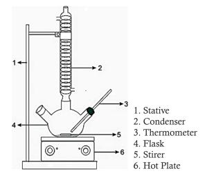
Figure 2. A set of refluxed apparatus
