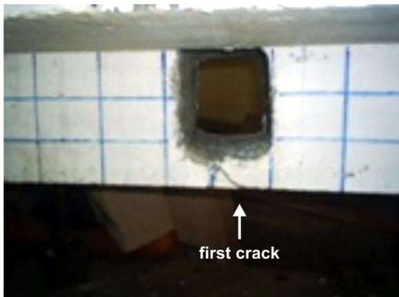
Gambar 14. Pola *first crack* BLKLB01
