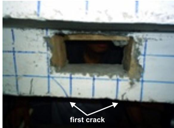
Gambar 15. Pola *first crack* BLKLB02
