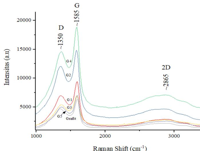
**Figure 5.** Raman spectroscopy results of graphene samples
