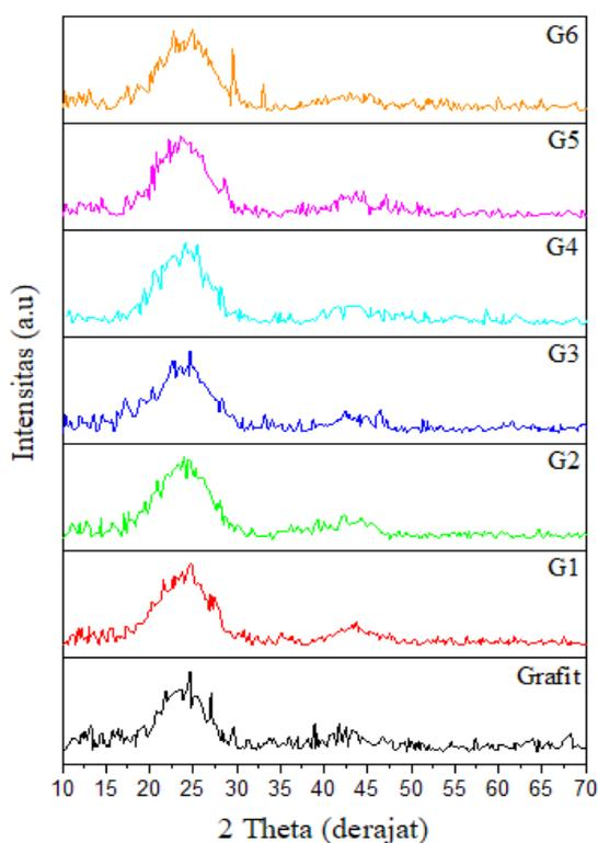
Figure 3. X-ray diffractogram for graphene samples
