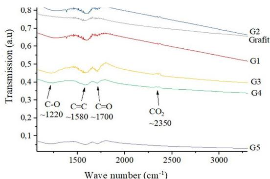
**Figure 4.** FTIR spectrum of graphene samples
