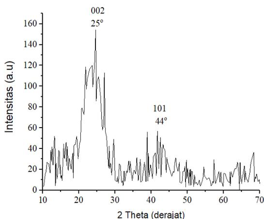
Figure 2. X-ray diffractogram of graphite
