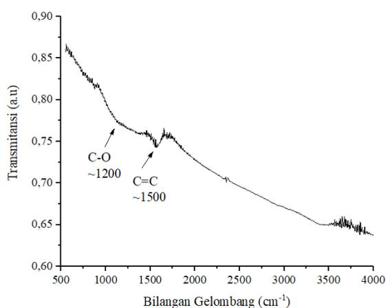
Figure 1. FTIR spectrum of graphite
