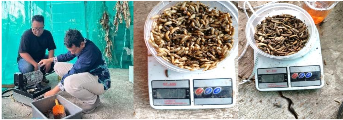
Figure 4. The process of drying maggots with a drying machine. The initial weight of 200 grams (center) becomes 114 grams (right)
