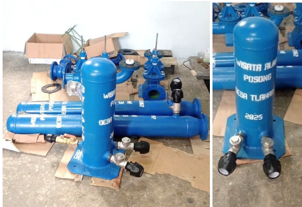
Figure 4. SmartHydra Twin Flow system combining hydraulic ram pumps with a stabilizer tube
