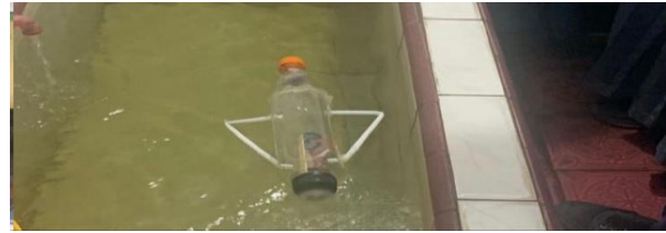
Figure 3. Miniature Ship Project During Testing Using Archimedes' Law Principle
