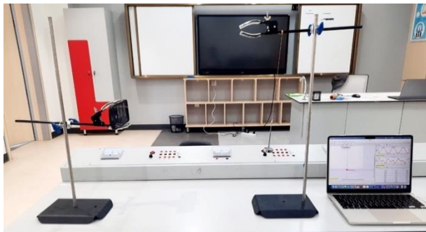
Figure 2. The setup for measuring the acceleration due to gravity using Tracker Video Analysis and Modelling.
