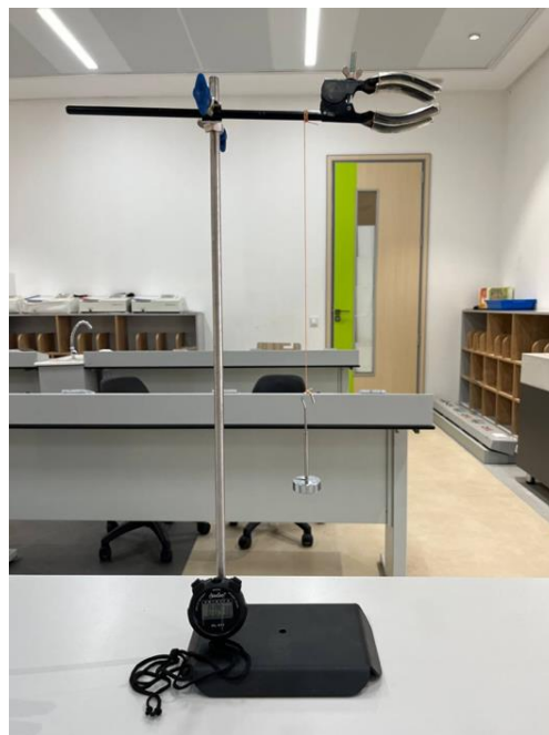
Figure 1. The setup is for a traditional method of measuring acceleration due to gravity.
