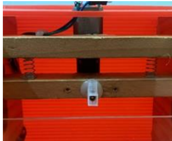
Figure 4. Wave generator system for producing water waves.
