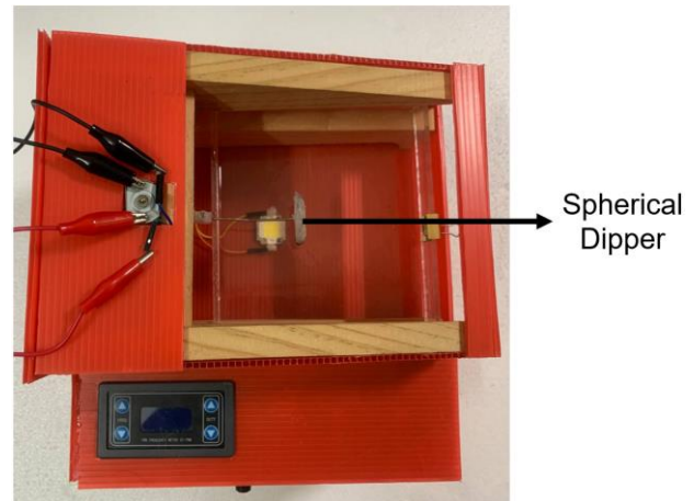
Figure 16. The spherical dipper generates two coherent sources for observing wave interference patterns.
