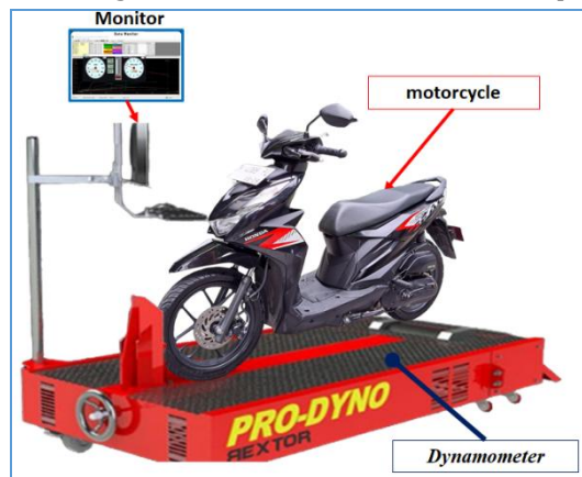
Figure 4. Vehicle performance test setup
