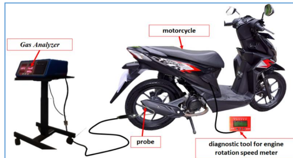
Figure 2. Vehicle exhaust emission test setup
