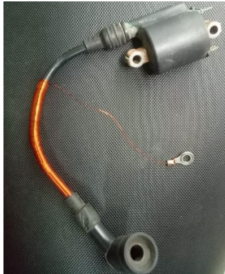
Figure 1. Groundstrap on spark plug cable
