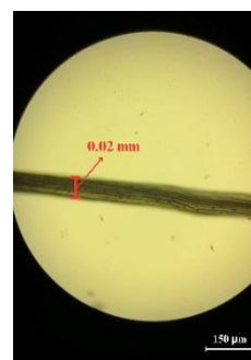
Figure 6. Micro Photograph of 7% Sisal Fiber
