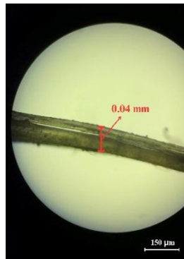
Figure 7. Micro Photograph of 10% Sisal Fiber
