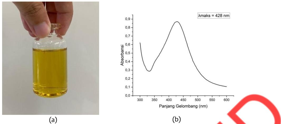
Figure 1. a) Synthesis Result of AgNPs; b) UV-Vis Spectrum of AgNPs
