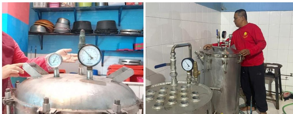
Figure 2. Pressure cooker and milkfish processing sterilization tool
