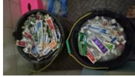
Gambar 1. Proses Perendaman Tube Pasta Gigi Sumber: Dokumentasi Peneliti, 2021
