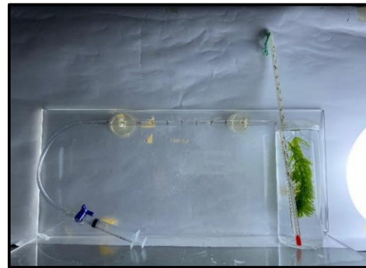
Figure 2. Modified Ingenhousz photosynthesis experiment kit
