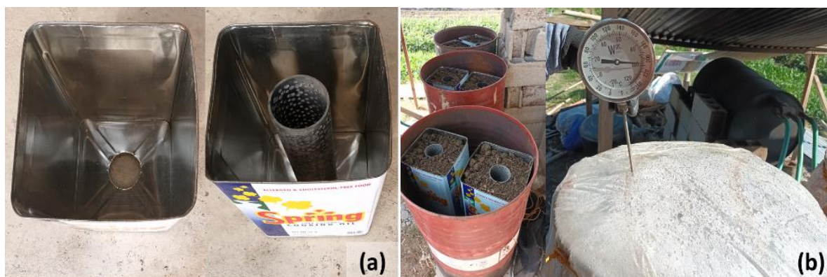
Figure 1. Materials used in the soil sterilization (a) A 16-liter capacity recycled vegetable oil can with a 2.5-inch diameter at the bottom and a perforated 3-inch diameter PVC pipe at the center, (b) a soil sample in a 200-liter capacity drum sterilized at 90-100 °C for 4 hours.
