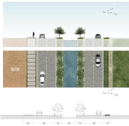
Figure 11 Existing Road Cross-Section
