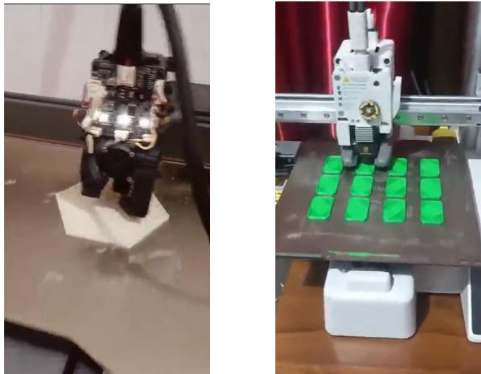
Figure 6. Process of printing tiles and tokens using PLA (Polylactic Acid) with the FDM (Fused Deposition Modeling) method
