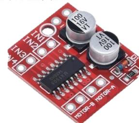
Gambar 4. MX1508 Driver Motor DC Dual 2V-10V 1.5A L298N
