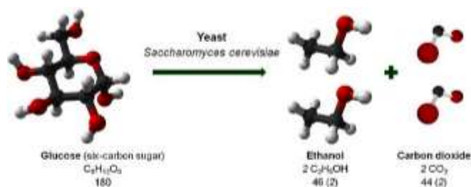
Figure 2. Conversion of Glucose into Ethanol and Carbon Dioxide by Yeast ( Bioenergy Research Group, n.d. )
