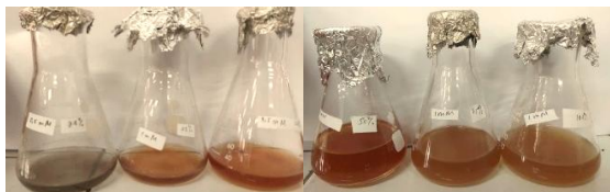
Figure 2. Silver nanoparticles' synthesis using bio-reductant of wuluh star fruit extract.
