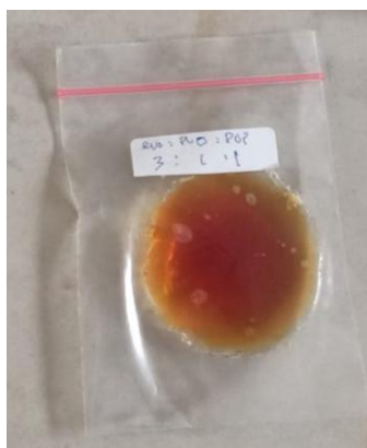
Figure 3. Visual observation of epoxidized palm cooking oil- polyvinyl chloride-dioctyl phthalate mixture after thermal treatment.
