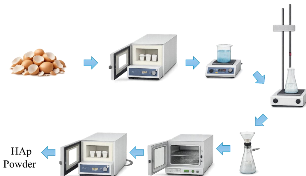
Figure 1. Schematic illustration of the HAp synthesis process using waste eggshell as the calcium precursor.
