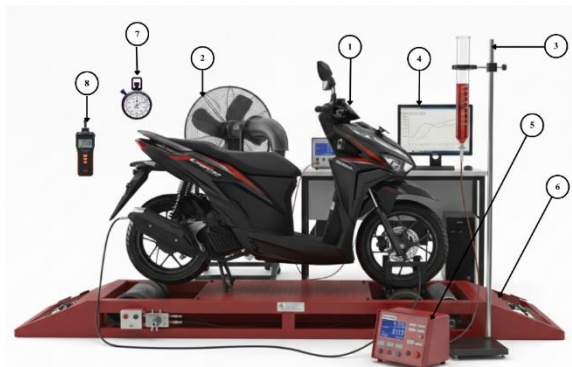
Figure 1. 2018 Vario 125cc motorcycle testing. (1) 2018 Honda Vario 125cc motorcycle (2) blower (3) measuring tank (burette) (4) display monitor dyno test (5) gas analyzer (6) chassis dynamometer (7) stopwatch (8) tachometer digital.
