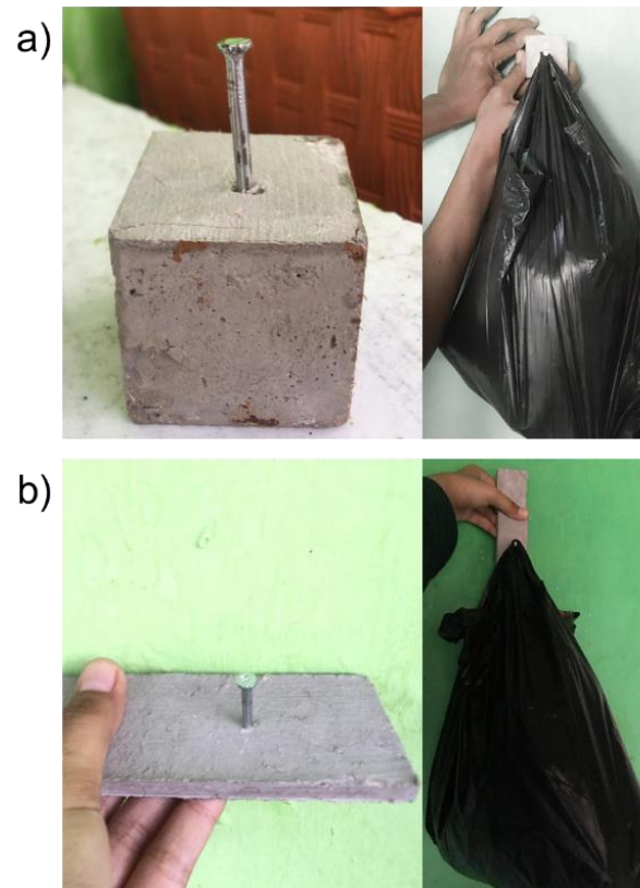
Figure 4. Nail embedded in the board (10% EFB) without breaking the board for a dimension of 5×5×5 cm (a) and 16×4×1 cm (b). The nail does not detach while weighing 4 kg weight.
