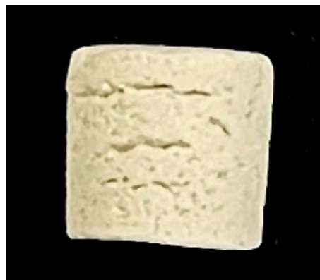
Figure 4. Cracks on the HA-Gel scaffold
