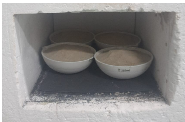
Figure 2. Calcination process of green mussel shell powder
