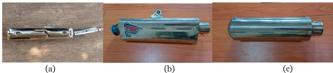
Figure 1. Exhausts (a) Standard, (b) Free-flow, (c) HPLPM Mod 2
