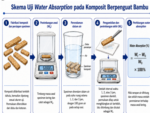
Figure 4. Schematic of the water absorption testing
