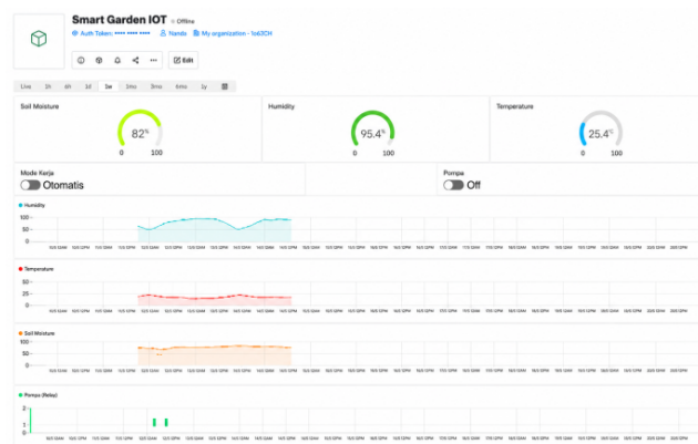
Figure 4. Blynk Cloud dashboard view for remote system monitoring
