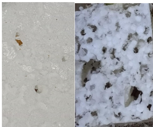
Figure 3. Styrofoam with holes due to being eaten by mealworms, and the condition of the styrofoam after 30 days of treatment
