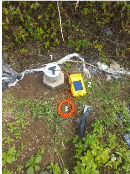
Figure 3. Microseismic Equipment (MAE Vibralog), 1) 3-Component MAE Sensor, 2) Digital Seismograph (Vibralog), 3) Digitizer to Sensor Connecting Cable
