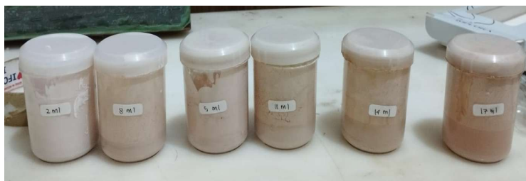
Figure 3. Betacyanin pigment-based wall paint.
