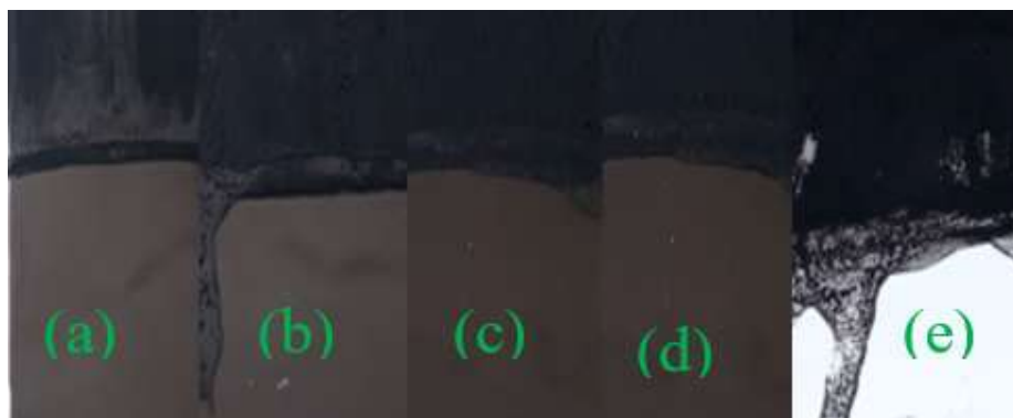
Figure 7. cElectrodes after electrophoretic deposition for 50 minute by applying different DC voltages
