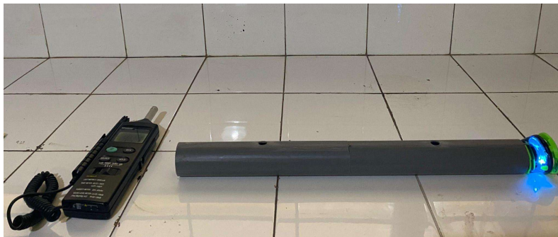
Figure 2. Simple Impedance Tube for Measuring Sound Absorption Coefficient.
