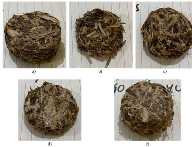
Figure 4. Composite sound absorber samples: (a) Sample A, (b) Sample B, (c) Sample C, (d) Sample D, (e) Sample E.
