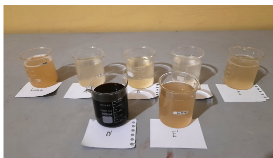
Figure 5. Documentation of wastewater samples and filtration results, with (left to right) waste 3, B3, C3, D3, A3 (back row), E3', and A3' (front row).
