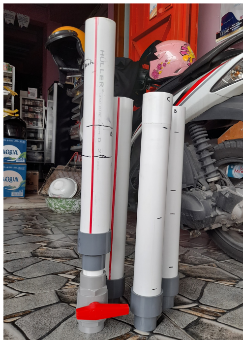
Figure 2. Domestic wastewater filtration device.
