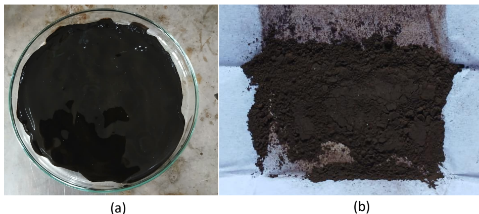
Figure 2. Nanoparticle samples (a) Iron sand synthesis sample after precipitation and (b) Green synthesis results of \text{Fe}_3\text{O}_4 nanoparticles.
