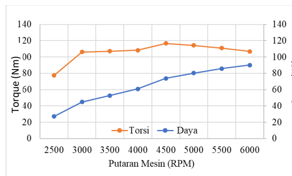
Figure 7. Power and Torque Graph of Magnetic Coil with a diameter of 0.35 mm
