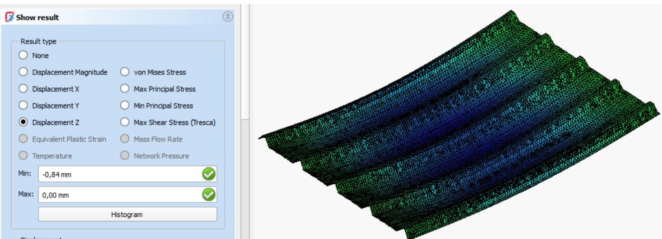
**Figure 6.** Simulation results of proposed trapezoidal corrugated roof
