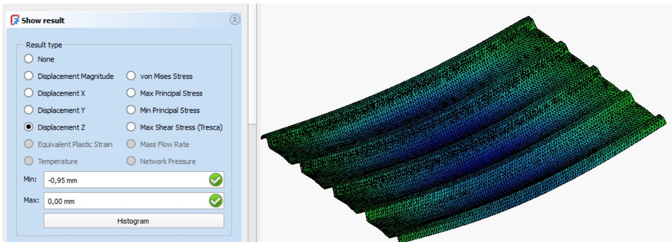
**Figure 5.** Simulation results of existing trapezoidal corrugated roof
