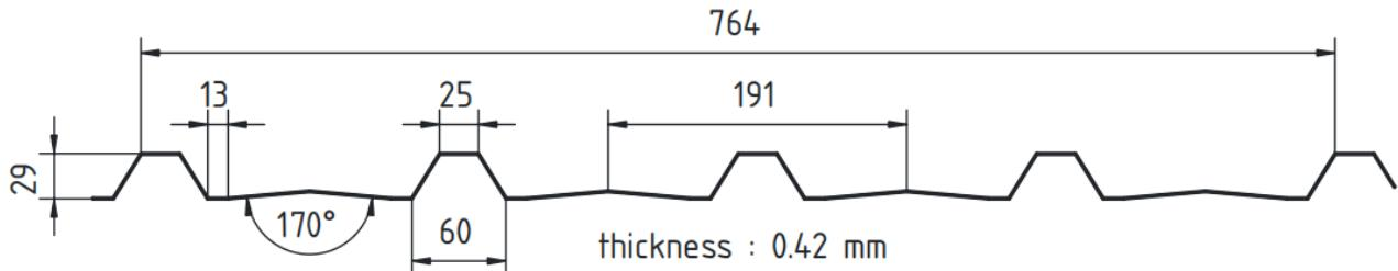
**Figure 3.** Existing cross-sectional geometry of trapezoidal corrugated roof
