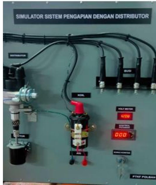
Figure 6. Installation of ignition simulation tool components
