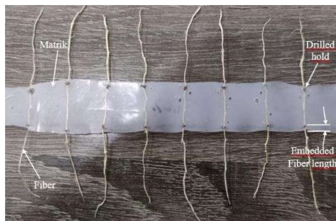
**Figure 2.** Specimen Test IFSS
