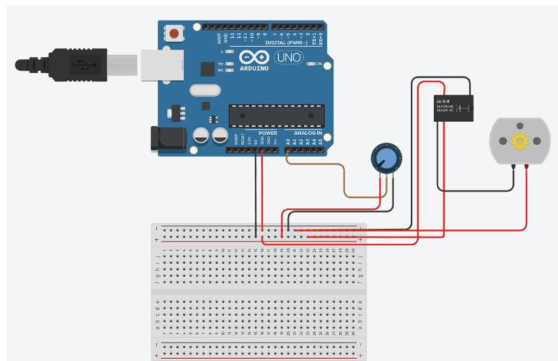
**Figure 2.** Schematic Diagram of Arduino-Based Automatic Irrigation System
