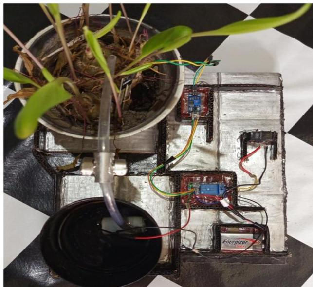
**Figure 3.** Arduino-based Automatic Watering Prototype
