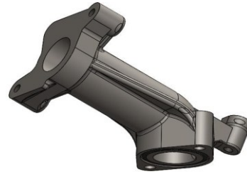
Figure 1. Geometry of the 120° intake manifold
