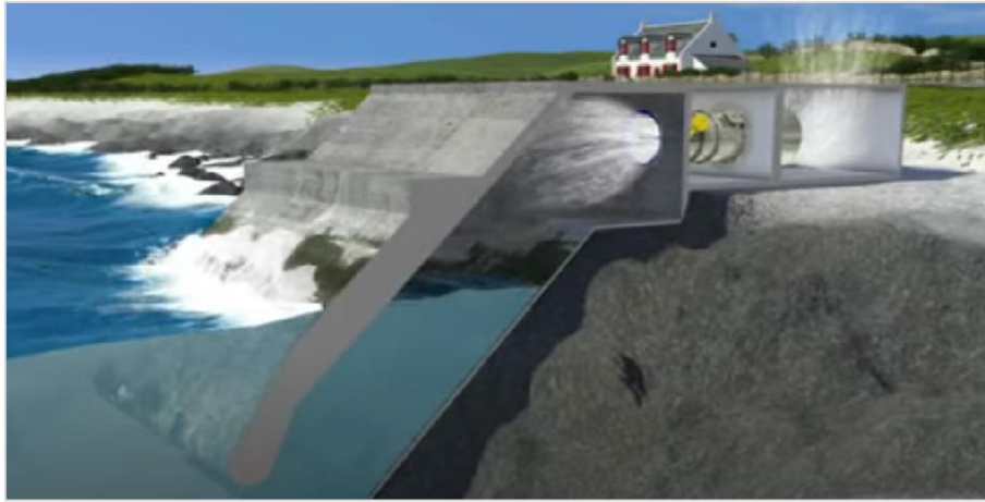
Figure 3. Concept of Oscillating Water Column [50]
