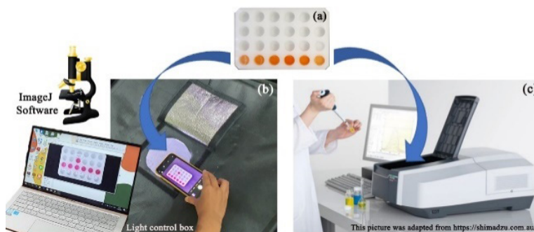
Figure 2. Experiment on the White Acrylic Well Plates (a), Determination of K_c by the alternative Colorimetric Analysis Method Using a Smartphone and a Light Control Box (b), and Standard UV-vis Spectrophotometry (c)
