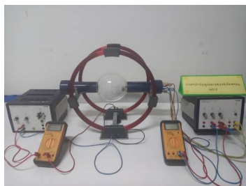
a. Specific Charge of the Electron Equipment (front view)
