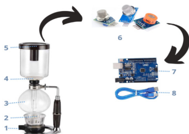
Figure 1. Coffee Maker Circuit Integrated with Arduino Gas Sensor
