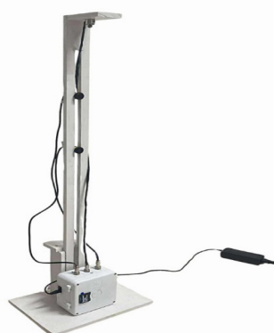
Figure 2. The Arduino-Based Motion-Timing Sensor: Experimental Setup
